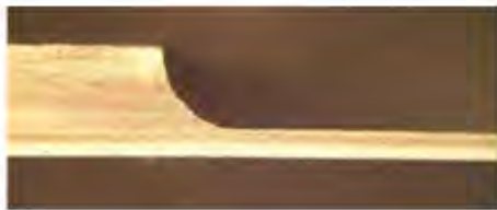
(b) Cross section of the micro-machined circular membrane
